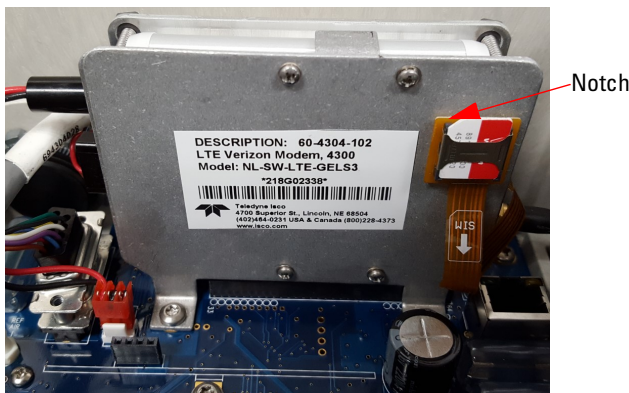
Figure 4: SIM card inserted into holder
