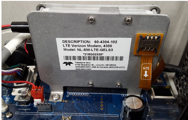
Figure 3: Location of the SIM card holder
